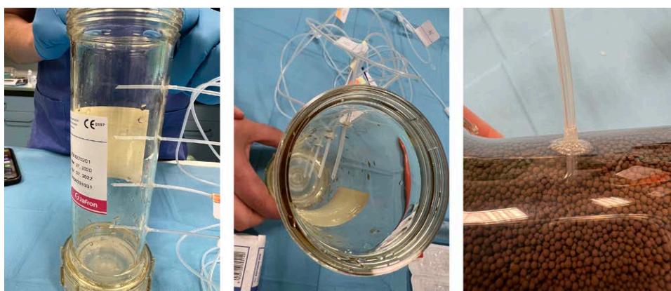
Figure 3. HA380-modified cartridge. The images in the left and in the middle show the modified cartridge emptied. The tip of the tubes was positioned in the center of the polycarbonate cylinder. The image on the right demonstrates the cartridge filled with sorbent material with a spherical shape (beads), and the position where the tube perforates the cylinder.
